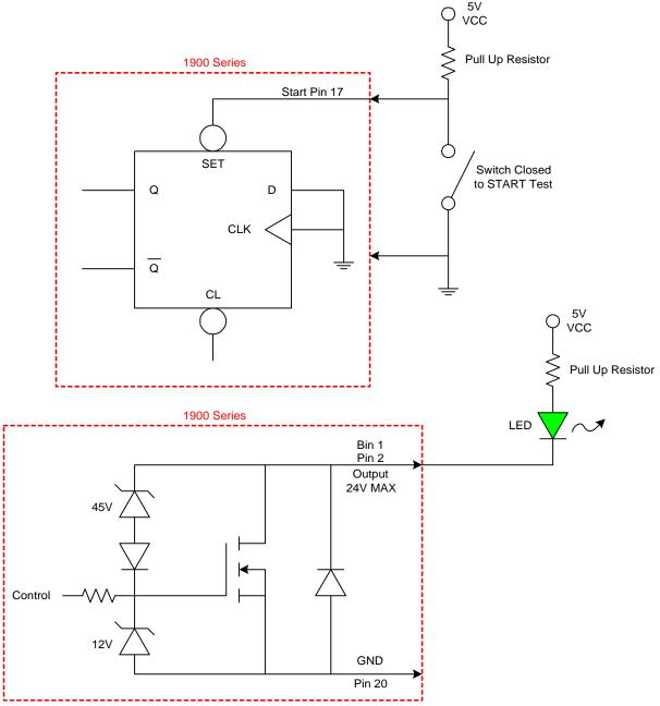
Figure 4.0: Switch & LED Connection
