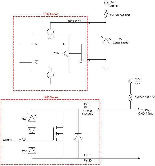
Figure 5.0: Connection to PLC
