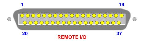
Figure 1: Remote I/O Pin Configuration
